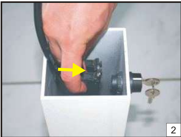
Fit the connector of the key contactor.
