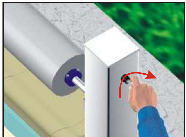
Run the driving shaft with the key and with the provided accessory (at the same time) activate the end-of-stroke adjustment until the shutter stops correctly (see figure 3). Perform this maneuver again until the required adjustment.
