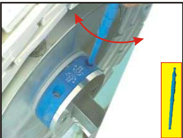
Run the driving shaft with the key and with the provided accessory (at the same time) activate the end-of-stroke adjustment until the shutter stops correctly (see figure 3). Perform this maneuver again until the required adjustment.
