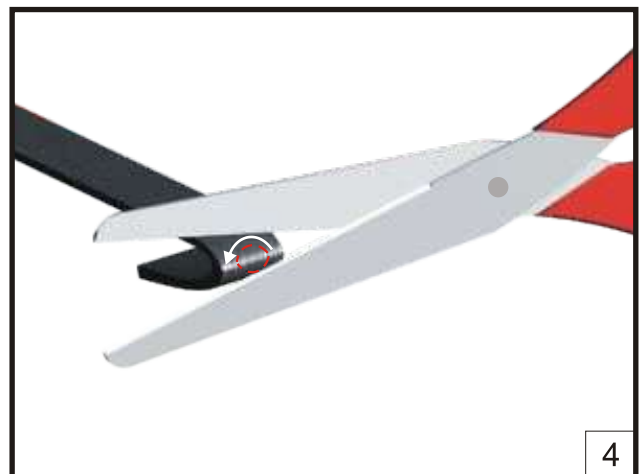
Bend the strap end and cut a half-disk in the center to make a circular hole.
