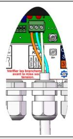
Connect the opening and closing contacts to the corresponding terminals. Common = 24VDC. 0Vdc terminal available if required to connect a wireless control system
