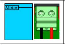
The red and black wires of the motor are connected to the terminal blocks according to the position of the motor in the pool
