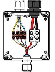
Junction box to be installed beneath edging tile (not supplied).
