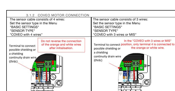
Recommended sensor cable: shielded 4-wire cable. Minimum cross-section 0.75 mm², max. length 50 m
