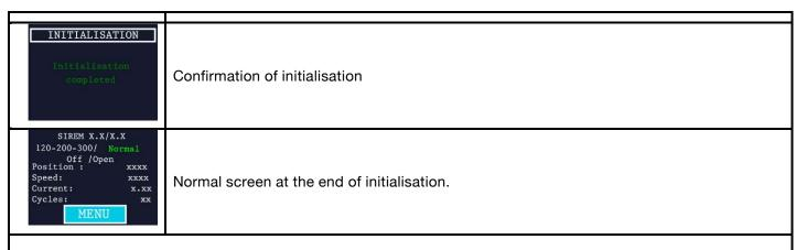
The speed of the "MANUAL" and "INITIALISATION" modes is reduced by 50% and is not the opening or closing speed after initialisation.
